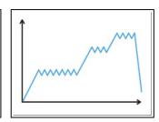
In the event of a fall, the tearing of the energy absorber webbing limits the impact force on the user. The lanyards are designed for users who weigh between 50 and 140 kg. The progressive tearing of the webbing reduces the deceleration on lightweight users.
