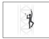
The ABSORBICA®-Y lanyards with two arms allow for continuous protection by successively detaching and re-attaching the two arms.
